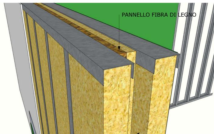
FINITURA ESTERNA CON PANNELLO ACQUAPANEL, INTONACO/RASATURA E TINTEGGIATURA ESTERNA
